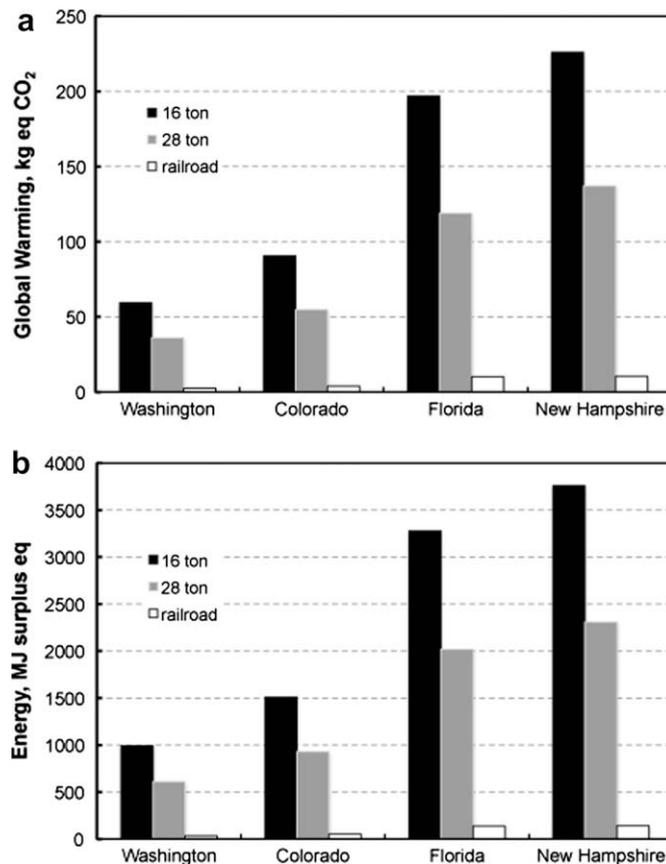
Fig. 5. a) Global warming emission in kg eq CO<sub>2</sub> for 250 of each type of containers (PLA, PET, PS) distributed by a 16- or 28-ton truck or railroad to WA, CO, FL and NH; b) non-renewable energy in MJ for 250 of each type of containers (PLA, PET, PS) distributed by a 16- or 28-ton truck or railroad WA, CO, FL and NH.
