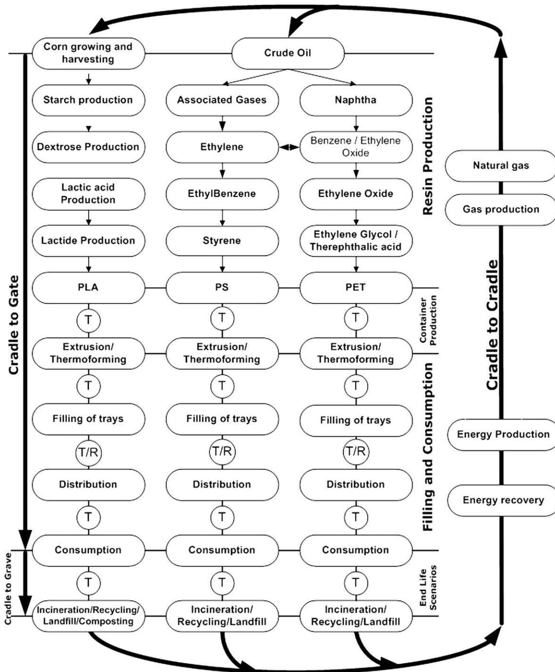
**Fig. 1.** Life cycle inventory flow chart for PLA, PET and PS thermoformed containers from cradle to gate, cradle-to-grave, and cradle-to-cradle. (T – transport, T/R – transport with refrigeration).
