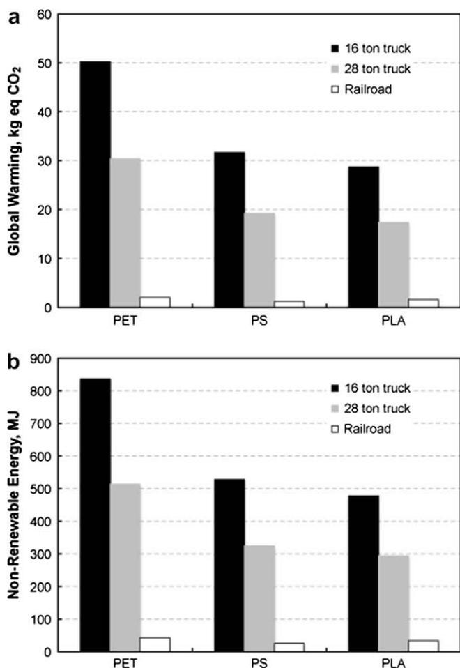
Fig. 4. a) Global warming emission in kg eq CO<sub>2</sub> for 1000 of each type of resins (PLA, PET, PS) distributed by a 16- or 28-ton truck or diesel locomotive; b) non-renewable energy in MJ for 1000 of each type of resins (PLA, PET, PS) distributed by a 16- or 28-ton truck or diesel locomotive.
