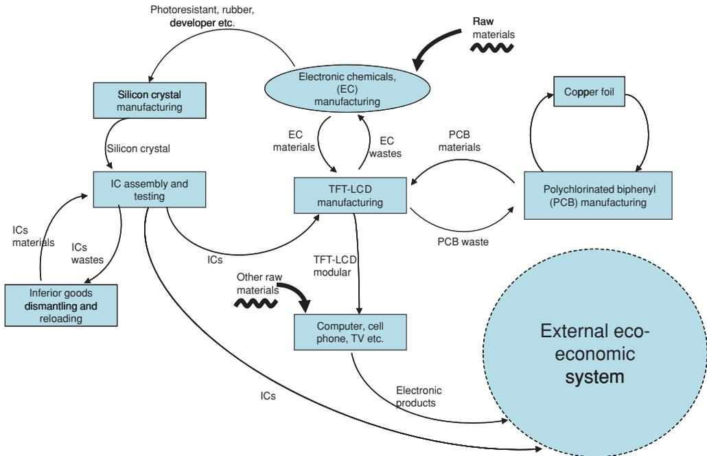
**Figure 5** Selected industrial symbioses in Suzhou Industrial Park. The variation in the thickness of the lines is an indication of the magnitude of the flows; the squiggly lines indicate the raw materials taken from nature outside the eco-industrial parks. IC = integrated circuit; TFT-LCD = thin-film transistor liquid crystal display; PCB = polychlorinated biphenyl.
