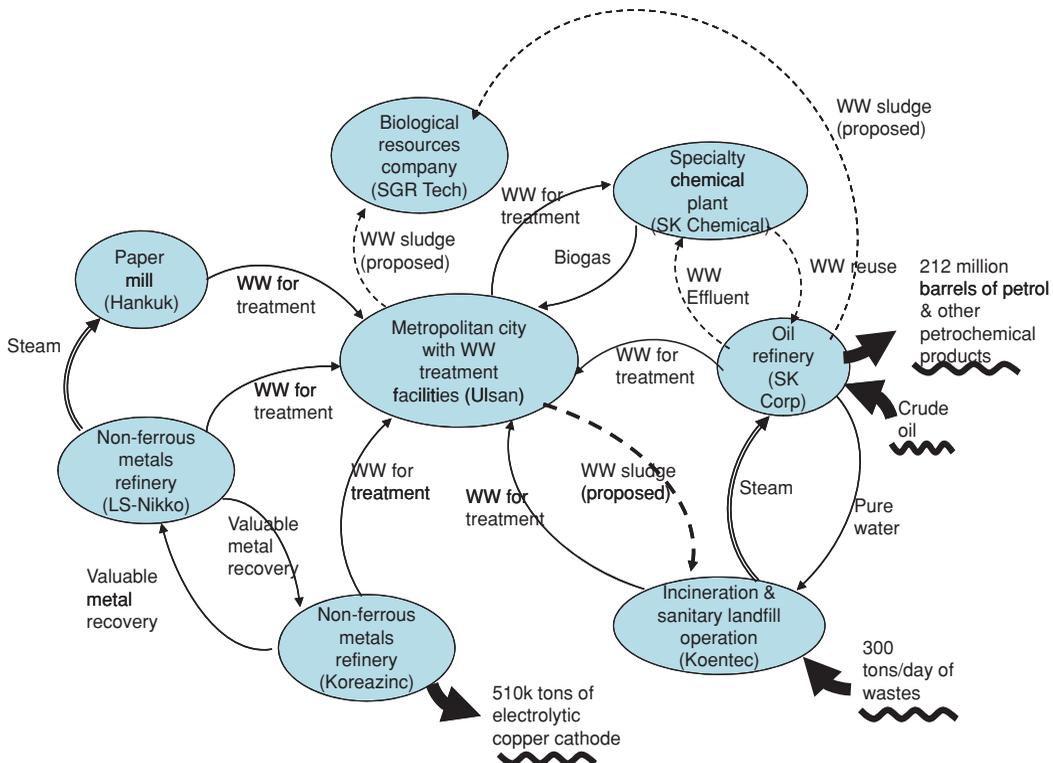
**Figure 9** Selected industrial symbioses in Ulsan industrial complexes, Korea. The variation in the thickness of the lines is an indication of the magnitude of the flows; the squiggly lines indicate the raw materials taken from nature outside the eco-industrial parks. WW = wastewater; k = thousand. Source: Based on the work of Park and colleagues (2008).
