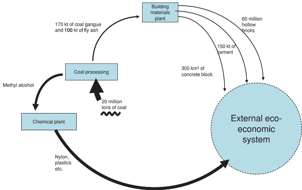
**Figure 3** Selected industrial symbioses in the Pingdingshan Coal Mining Group. The variation in the thickness of the lines is an indication of the magnitude of the flows; the squiggly lines indicate the raw materials taken from nature outside the eco-industrial parks. kt = kilotonne; km = kilometer. Source: Based on the work of Long and Zhang (2009) as well as Pingmei's Web site ([www.pmj.com.cn](http://www.pmj.com.cn)).
