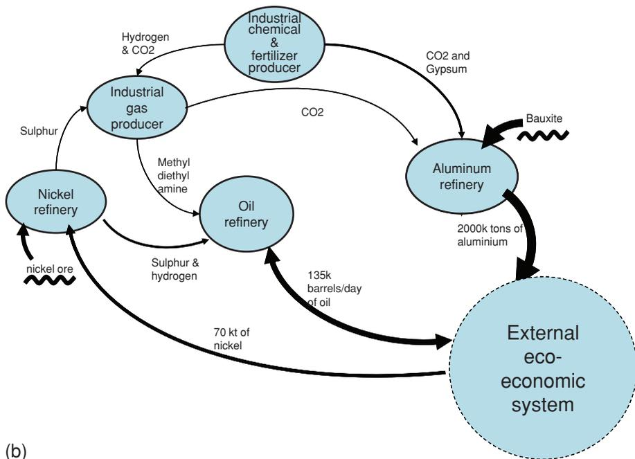
**Figure 8** (A) Selected industrial symbioses in Kwinana, Australia (1) with focus on titanium dioxide. (B) Selected industrial symbioses in Kwinana, Australia (2) with focus on nickel. The variation in the thickness of the lines is an indication of the magnitude of the flows; the squiggly lines indicate the raw materials taken from nature outside the eco-industrial parks. kt = kilotonnes; k = thousand.
