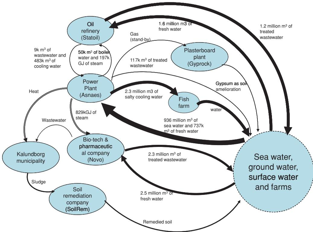
**Figure 7** Selected industrial symbioses in Kalundborg, Denmark. The variation in the thickness of the lines is an indication of the magnitude of the flows. m = meters; k = thousand; GJ = gigajoules; CO<sub>2</sub> = carbon dioxide.
