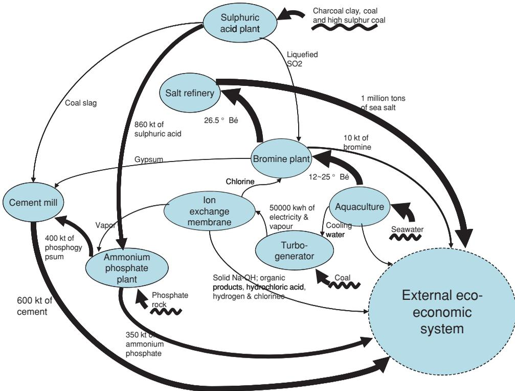
**Figure 4** Selected industrial symbioses in Lubei Industrial Park. The variation in the thickness of the lines is an indication of the magnitude of the flows; the squiggly lines indicate the raw materials taken from nature outside the eco-industrial parks.  $\text{SO}_2$  = sulfur dioxide; kt = kilotonne; kwh = kilowatt hour; NaOH = sodium hydroxide.
