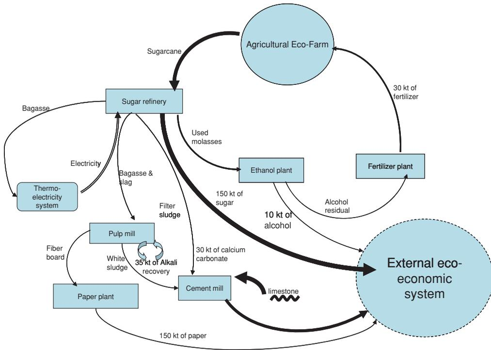
**Figure 2** Selected industrial symbioses in the Guitang Group, Guigang City. The variation in the thickness of the lines is an indication of the magnitude of the flows; the squiggly lines indicate the raw materials taken from nature outside the eco-industrial parks. kt = kilotonne.
