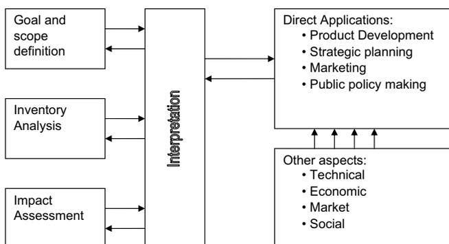
Fig. 2. Phases and applications of LCA adapted from ISO 14040:1997 [4].
